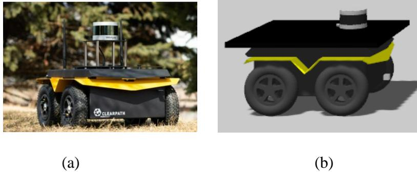
*Figure 8: a) 3D view of Jackal with ZED2 camera and VLP-16 lidar[13], b) simulated 3D view of Jackal with ZED2 camera and VLP-16 lidar*
